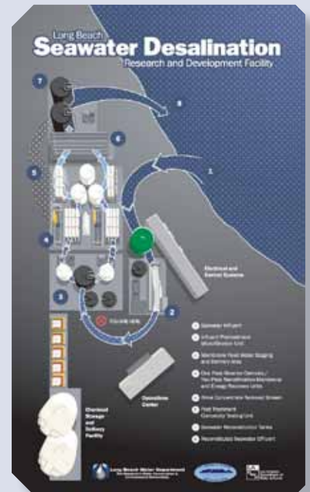
Schematic of the Long Beach Seawater Desalination Facility
